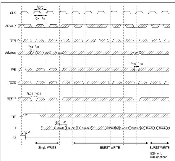
Notes: 1.  $\overline{\text{CE3}}$  and  $\overline{\text{CE2}}$  have timing identical to  $\overline{\text{CE1}}$ . On this diagram, when  $\overline{\text{CE1}}$  is LOW,  $\overline{\text{CE3}}$  is LOW and CE2 is HIGH. When  $\overline{\text{CE1}}$  is HIGH,  $\overline{\text{CE3}}$  is HIGH and CE2 is LOW.
