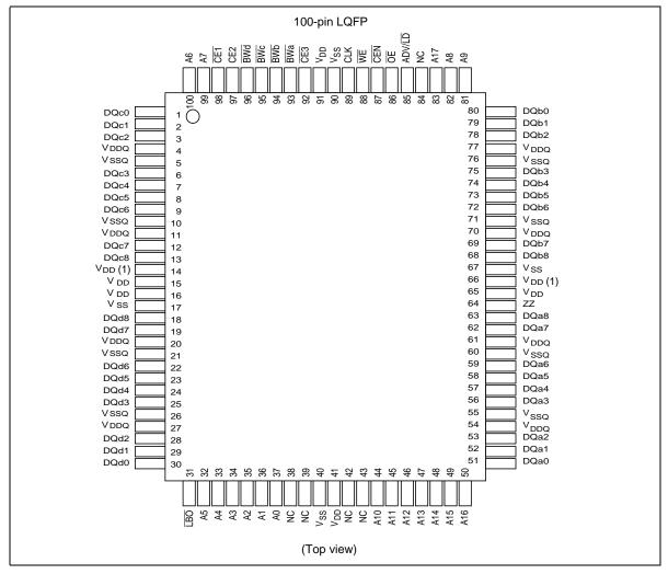
Note: Pins 14 and 66 are not  $V_{\scriptscriptstyle DD}$  Supply, but have to be connected  $V_{\scriptscriptstyle DD}$ .
