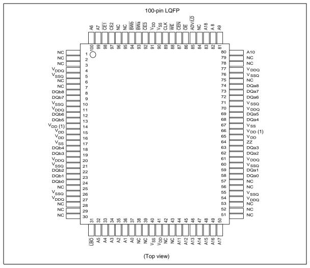
Note: Pins 14 and 66 are not  $V_{\rm DD}$  Supply, but have to be connected  $V_{\rm DD}$ .
