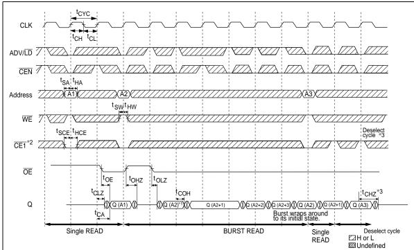
Notes: 1. Q (A2) refers to output from address A2. Q (A2 + 1) refers to output from next internal burst address following A2.
